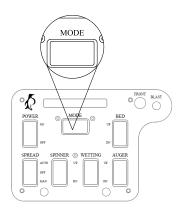
The Mode selection switch is centered under the LCD display. The switch is a 3 position momentary type that allows the user to "scroll" through the available display modes. As you scroll through the available modes, the display will briefly read "MODE XX", where "XX" is the corresponding mode number. The Mode information will then be displayed.
