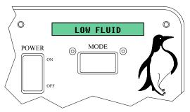
This warning indicates that the hydraulic fluid in the reservoir tank is low. The display will flash "LOW FLUID" and create an audible beep. Also, all spreader functions will be disabled. The bed and plow functions will remain in operation as long as there is some fluid in the tank. If the fluid level is low, immediate maintenance is recommended. To override a faulty low oil alarm and enable spreader functions, turn to MODE 8 with the spreader switch off and hit the blast switch
