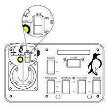
The Bed thumb-controller is located on the Joystick face (lower right). The rocker switch directs bed movement up and down at normal speed. To lower the bed at a faster rate push the rocker switch forward and press the Down Fast button (red push button on the right side of the Joystick) at the same time.
