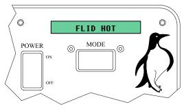
This warning indicates that the temperature has exceeded the maximum recommended operating temperature (default is 150°F). The control box will produce an audible beep and the display will flash "FLUID HOT". The current hydraulic fluid temperature can be displayed by scrolling to LCD MODE 10 on the main menu. Immediate maintenance of the truck is recommended.
