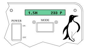
Displays the distance traveled in miles and material usage in pounds for each trip. It can be reset by turning the spreader switch off and hitting the blast button.
