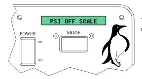
This warning indicates that hydraulic pressure has exceeded the maximum measureable pressure (2715PSI) while in Mode 9.
