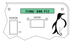
Displays the hydraulic pressure in pounds per square inch (PSI). High pressure sensor readings are on the left while a differential pressure reading is on the right (Main pressure—Pressure after auger/conveyor motor)
