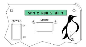
Displays the current setting for the spinner, auger, and wetting motors.
