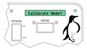
Used for gaining access to the calibrations. Access by pressing the blast button while the spreader switch is in the off position, enter the 4 digit pass code using the plow switch, then press the blast button again.
