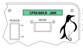
Spreader Jam will cause an Audible beep and the control box will flash "SPREADER JAM". This Indicates that Hydraulic pressure has exceeded the maximum (default is 2500PSI), and no material is being ejected by the spreader. It may be caused by a material jam at the auger/conveyor or a quick disconnect to any of the drive motors may not be connected.
