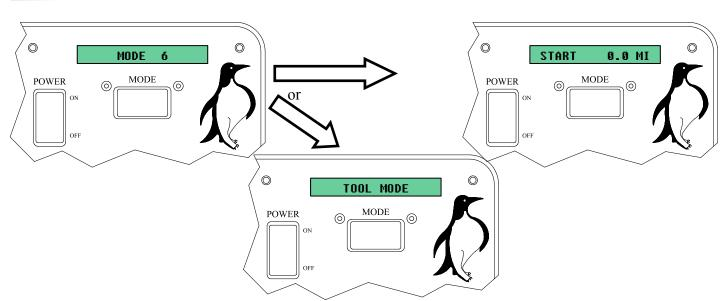
This position differs based on the spreader setting. In manual this is "**TOOL MODE**", allowing hydraulic tools to be run off the Pengwyn manifold without nuisance temperature and pressure alarms. This is described in detail below. With the spreader in automatic, this is no applicable function. If the spreader is switched off, this mode may be used for distance measuring feature in **miles**. Use the blast button to Start/Stop measuring.
