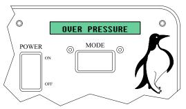
This warning indicates that hydraulic pressure has exceeded the maximum measureable pressure (2715 PSI), while hydraulic motors are not engaged (i.e. Spread switch is in the off position or in Auto at 0MPH). This condition can occur when a hydraulic pump controlled by a manual switch is put into a deadhead condition.
