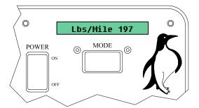
Displays the current spreading rate of the truck in lbs. of material per mile.
