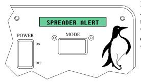
If there is an audible beep and the control box display flashes "SPREADER ALERT", material load on the auger has dropped below the preset minimum (set during calibration). If Automatic vibrator connection is installed it will be triggered as well. Spreader Alert indicates that there has been a reduction of the load on the hydraulic drive motor. Generally, this is caused when the spreader is running out of material. Other causes include:
