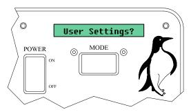
Used for gaining access to settings that do not require a pass code. These settings include turning on/ off counterbalance and broom mode. It also has the option to turn on speed simulation from 0-60 MPH in 5 MPH increments. This can be used to simulate automatic while the truck sits still. Press the blast switch to enter user settings and also use blast to exit and save any changes.
