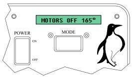
If the Fluid Temperature goes above a factory set, non-adjustable limit of 160° F, Pumps are shut down, an alarm sounds, "MOTORS OFF XXX°F" is displayed (where XXX is the oil temperature), and valve control is suspended. Once hydraulic oil temperature falls below 160°F function can be regained by turning spreader switch to the OFF position. Immediate maintenance of the truck is recommended.
