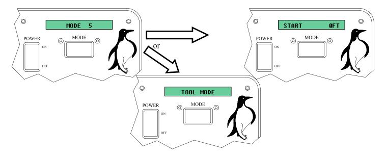
This mode differs based on the spreader setting. In manual this is "TOOL MODE", allowing hydraulic tool to be run off the Pengwyn manifold without nuisance temperature and pressure alarms. This is described in detail below. With the spreader in automatic, there is no applicable function. If the spreader is switched off, this mode may be used for the distance measuring feature in **feet**. Use the blast button to Start/Stop measuring.
