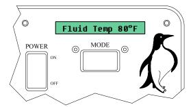
Displays the hydraulic fluid temperature in degrees Fahrenheit.
