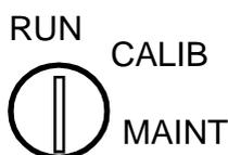
The programming and maintenance keyswitch has three settings. They are run, calibrate, and maintenance. **RUN** is at 12:00, **CALIB** is at 1:30, and **MAINT** is at the 3:00 position. Each setting will be discussed in more depth where they apply.
