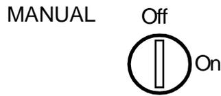
The manual lockout keyswitch position determines whether the system's manual control of the auger and/or spinner is available. If the key is in the off position, no power will be sent to the auger/spinner coils when the spreader switch is in **MANUAL**.
